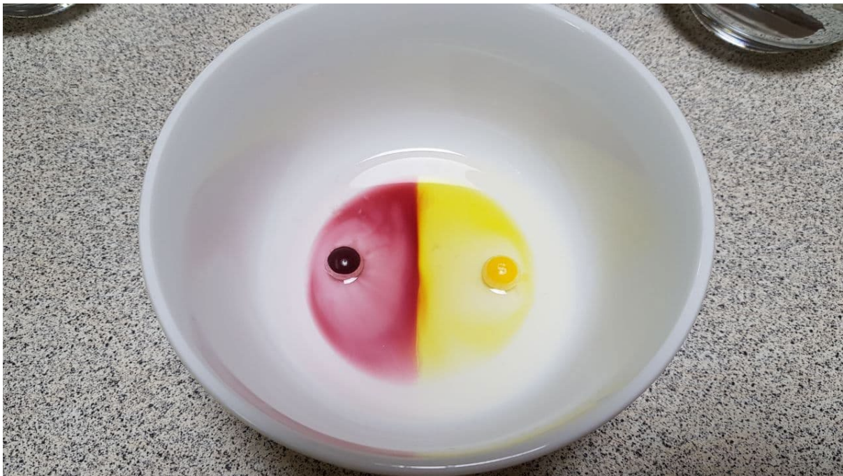
Figure 1. The sugar/dye will diffuse from areas of high concentration to areas of low concentration. A boundary is formed where the colours meet because the sugar/dye concentrations will be similar and they therefore tend not to mix
